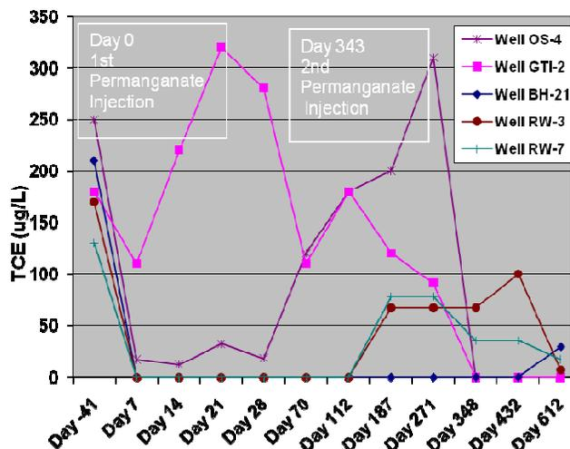
In April 2009 (Day 343), a second injection of 6,600 gallons of permanganate was injected into off-site well OS-4 and three other wells. An immediate reduction in TCE in well OS-4 from over 300 µg/l to non-detectable was monitored after this injection. Overall, the TCE plume has been reduced by over 95% in size. The map below illustrates the size of the TCE plume before and after treatment.
