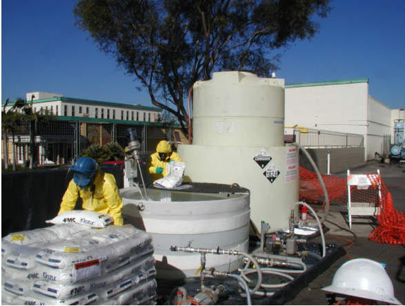
FIGURE 7. Mixing of persulfate solution.
