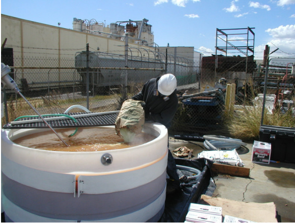
FIGURE 9. Mixing of ferrous sulfate into solution.
