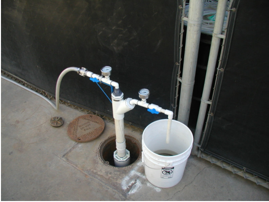
Figure 11. Well head injection apparatus.
